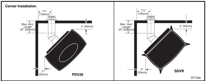
Fig. 4 Corner installation minimum clearances.
